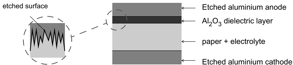
Figure 3.13 Electrolytic capacitor construction
